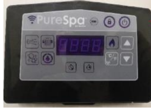
PureSpa Greywood, Greystone ve Jet&Bubble Deluxe Spa küvetinin kontrol paneli
