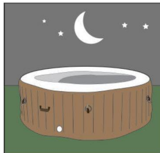
At night and at lower temperatures, the air automatically contracts, which makes the spa tub seem less sturdy. The spa tub is not leaking!
